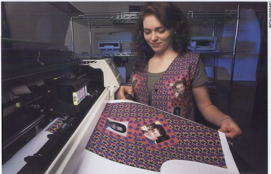
Corvallis employee Dianne Hodnett prints a pattern on cloth with an HP DesignJet 750C large-format printer. The cloth can be used to make a vest like the one she is wearing.
